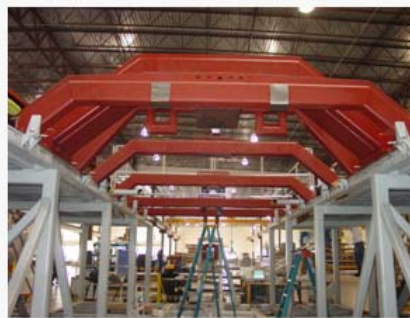
Other Beams used to locate Components in Design Coordinate System Relative to Base Fixture
