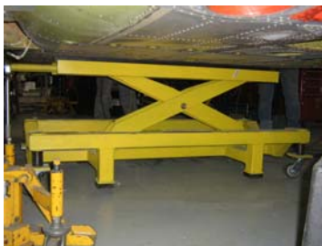
H-60 Scissor Floor Jacks Installed
