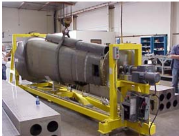
Tailcone Refurbishment Fixture with Tailcone Loaded
